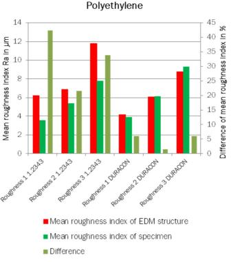
Comparison of reproduction of surface details between 1.2343 tool alloy and DURACON® 45M (Study of Fachhochschule Schmalkalden, picture left and diagram on the right).
