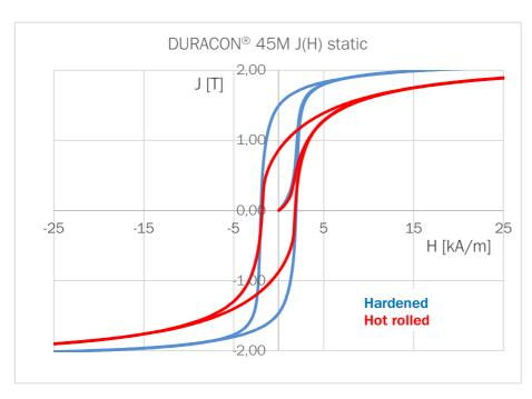
DURACON® 45M is ferromagnetic and combines a high saturation flux density and a moderate coercivity with excellent mechanical toughness. Besides the already mentioned option of inductive heating, this special combination, together with the good corrosion resistivity, could be of interest for some special applications. The diagram shows an example of static J(H) loops bevor and after hardening, measured at a rod of 10 mm diameter and a length of 90 mm.
