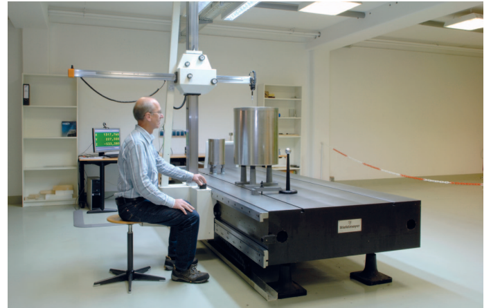
Figure 12: 3D measuring table for mechanical measurement
