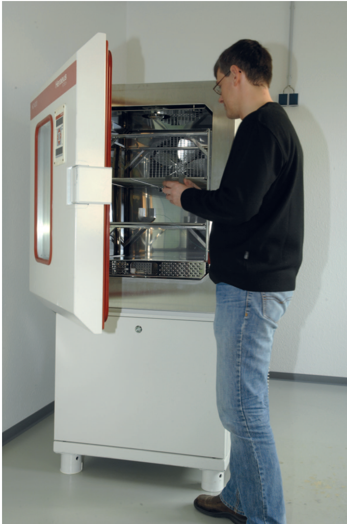
Figure 14: Measuring cabinet for temperature change and humidity tests.
