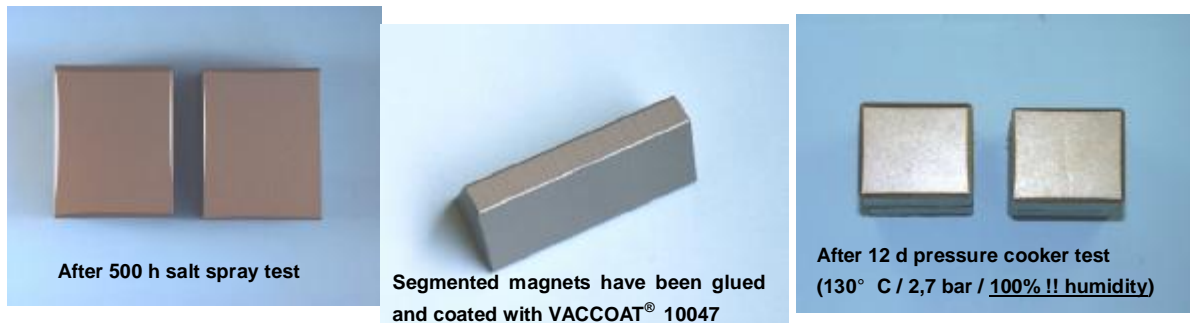
Fig. 7a Salt-spray test DIN 50021 and HAST (130°C; 2,7 bar 100% moisture)
