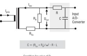
Condition for value of R: RB <<R<<IZI of converter; typical value R = 1 k $\Omega$ Typ. C values: 150 ... 300 nF
