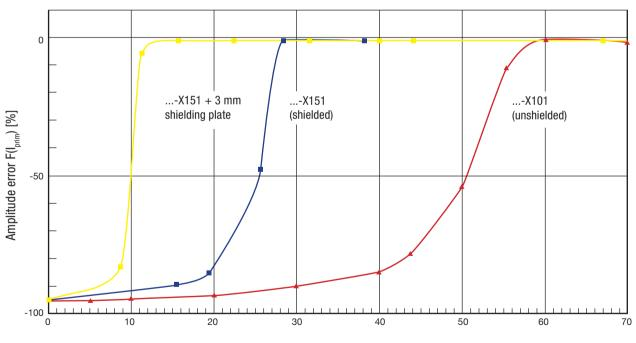
Sensitivity of E4624-X101/151 for DC magnetic fields \$\$ Magnet: VACOMAX® 65 x 65 x 35 mm \$\$
