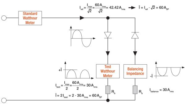
DC TOLERANCE TEST ACCORDING TO IEC 62053-21, -23
