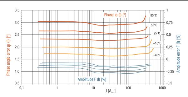
Fig. 9: 60 A with DC Tolerance, T60404-E4624-X121/-X171
