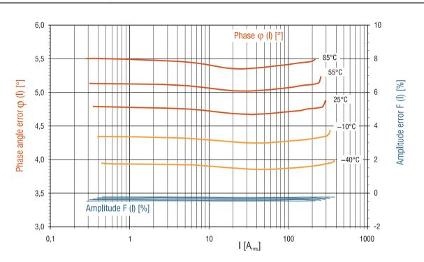
Fig. 5: 100 A with DC Tolerance, T60404-E4626-X101/-X501/-X151
